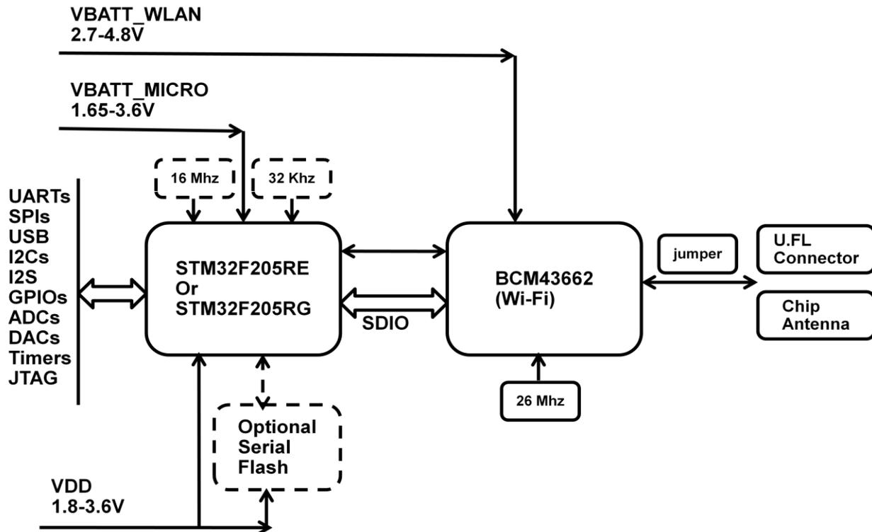
RZ707MS Module consists of two main components: an ARM Cortex-M3 based 32-bit microcontroller that runs Em-Fi Software and Broadcom BCM43662 Wi-Fi device. It also includes an optional serial Flash (1MB or 2MB), an on-board chip antenna and a u.FL connector for optional external antenna.
