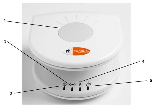
Figure 2—Front View of the Video Flex 2825 Wireless Multimedia Router
