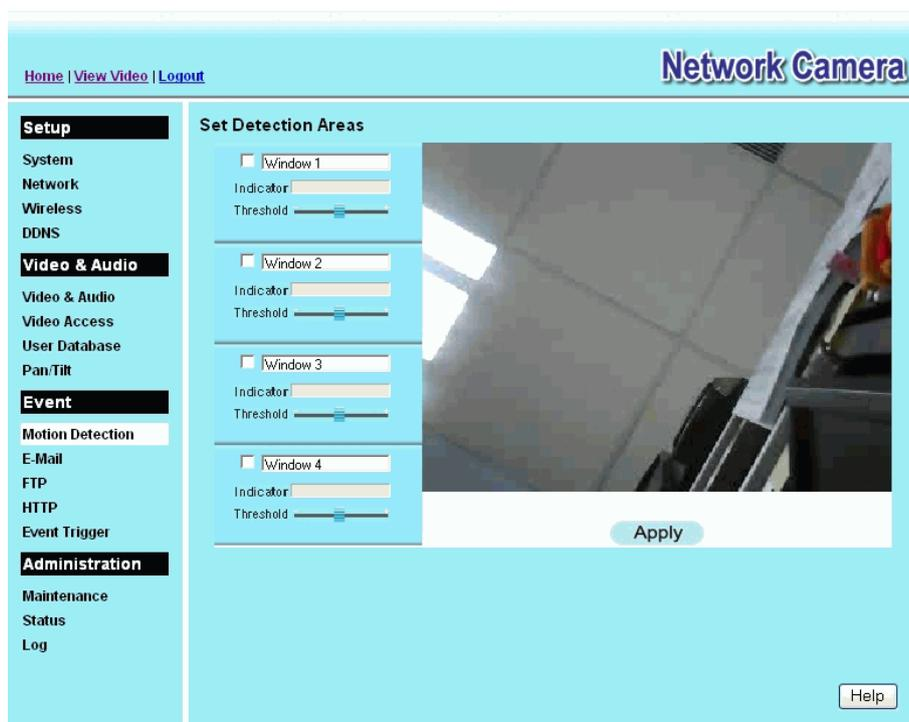
Figure 23: Motion Detection
