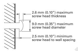
**Note**: If possible, mount the gateway to concrete, masonry, a wooden stud, or some other solid wall material. Use anchor bolts if necessary (for example, if you mount the unit on drywall).
