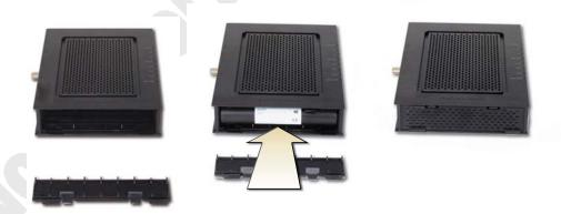
3. Set the battery cover into the bottom of the gateway and press down on the upper two locking tabs, and then push the cover shut until the tabs snap into place.
