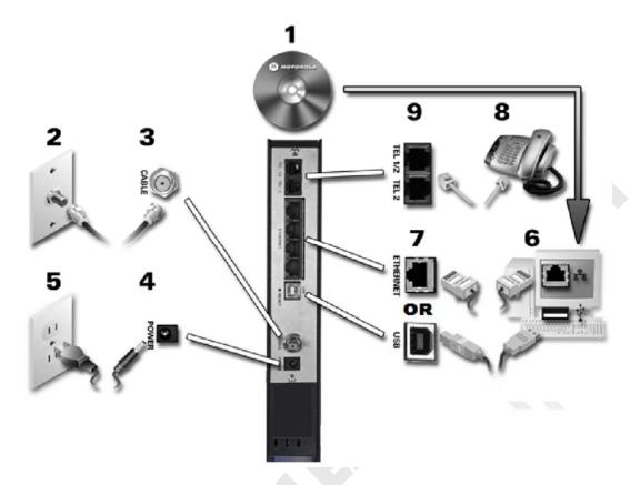
Figure 2 – SVG2501U Installation
