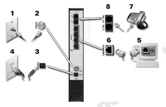
Figure 1 – SVG2501 Installation
