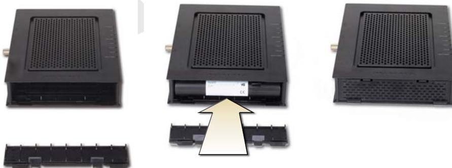
3. Set the battery cover into the bottom of the gateway and press down on the upper two locking tabs, and then push the cover shut until the tabs snap into place.
