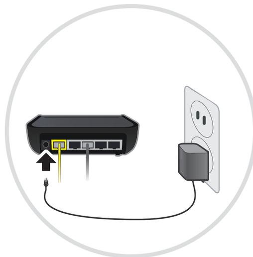
Plug the Router's power supply into the Router and a power outlet.
