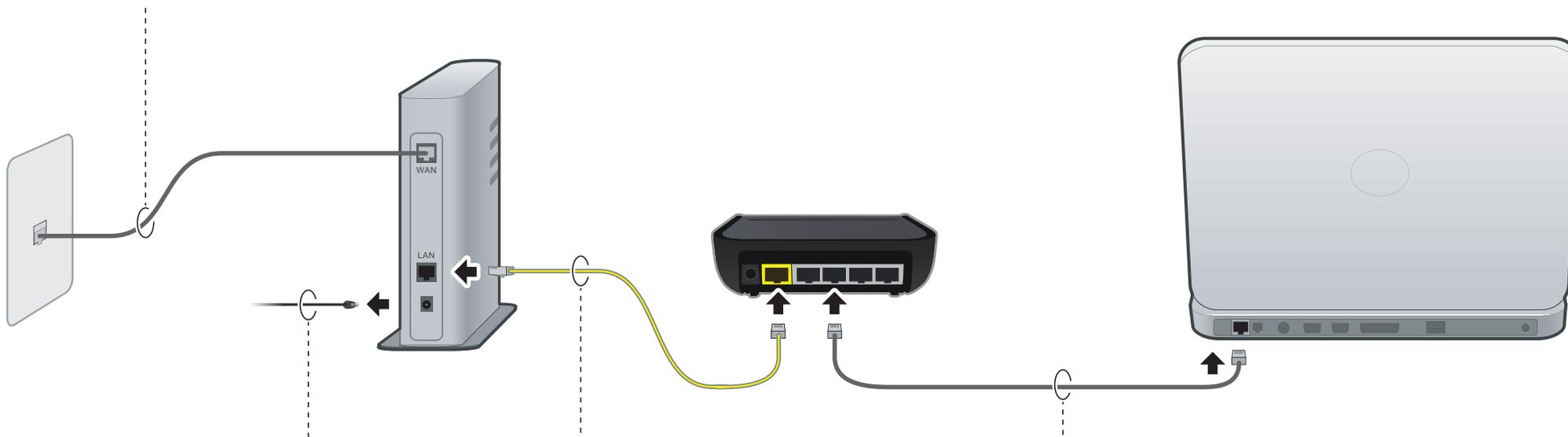
**[2]** Remove the power cord from your DSL or cable modem.
