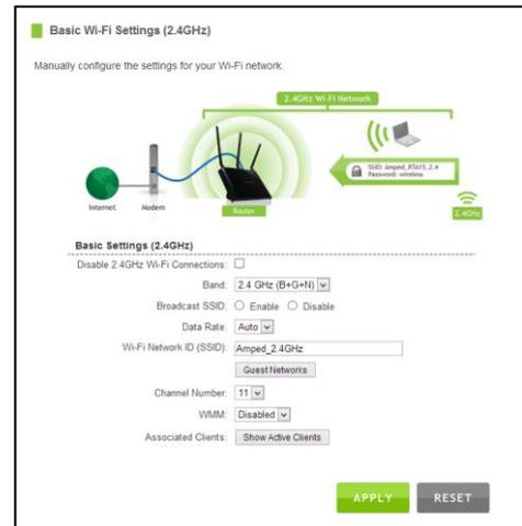
Channel Number: Wi-Fi networks operate on specific wireless channels. Some network channels may have more interference than others. If your performance is unstable, try a different channel number. If you are using a repeater with this network, it is recommended you set a static channel, instead of using "Auto."
