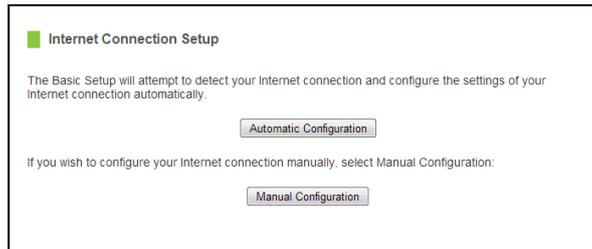
More advanced users may choose to configure their connections manually by selecting Manual Configuration. DSL users may require additional login information. Select the appropriate connection type and enter the required information.
