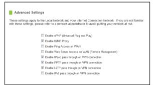
connection. With UPnP enabled, network devices may change security settings within the Router's firewall to allow access over the Internet. By default, UPnP is disabled to avoid exposing your network to security issues.
