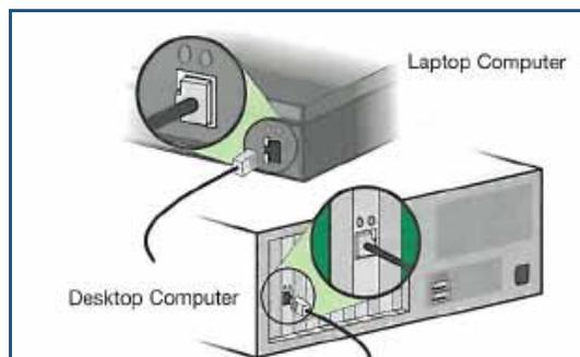
Figure 6. Connecting the Gateway to the a Laptop or Desktop Computer
