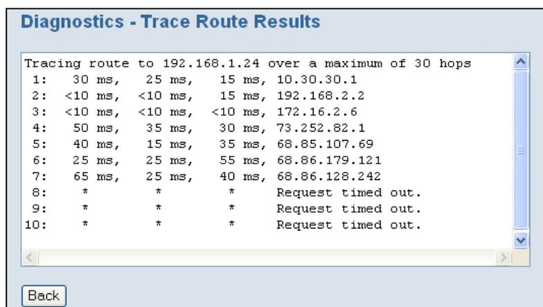
Figure 52. Example of Results for Trace Route
