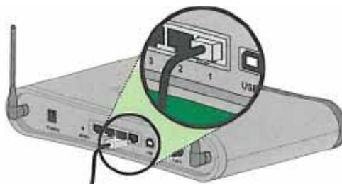
**Figure 5. Connecting to a LAN Port on the Gateway Rear Panel**
