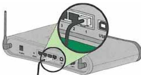
**Figure 5. Connecting to a LAN Port on the Gateway Rear Panel**
