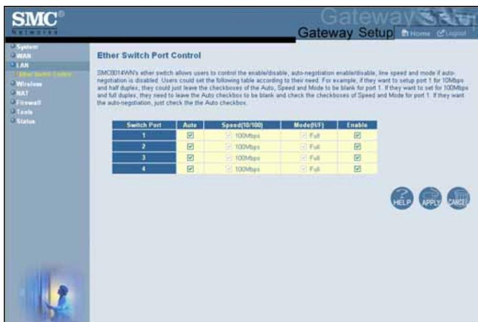
Figure 27. Ether Switch Port Control Menu
