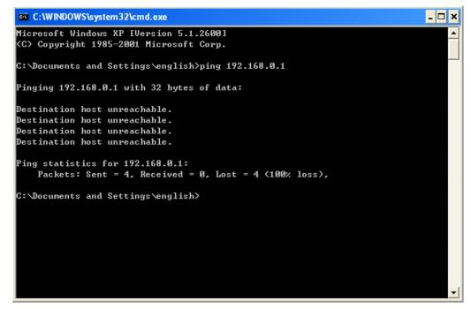
Figure 3-2 Failure result of Ping command
