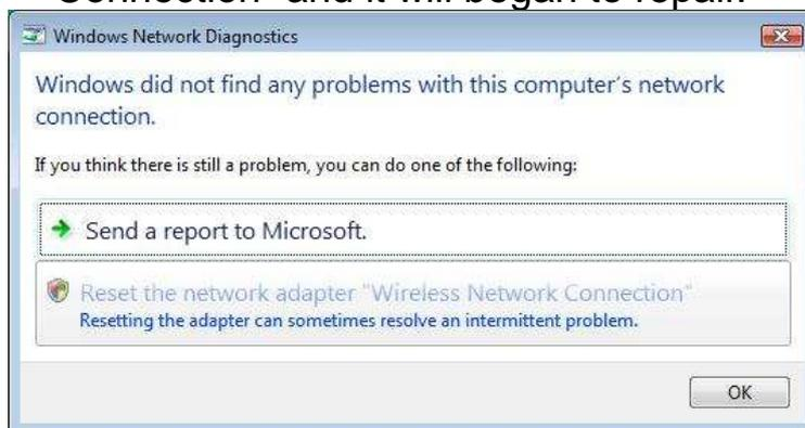
3. If you use Local Area Connection to connect the Router, please click Network and Sharing Center > Manage network connections > Local Area Connection > Diagnose, do the step 1 and following the message to repair it.
