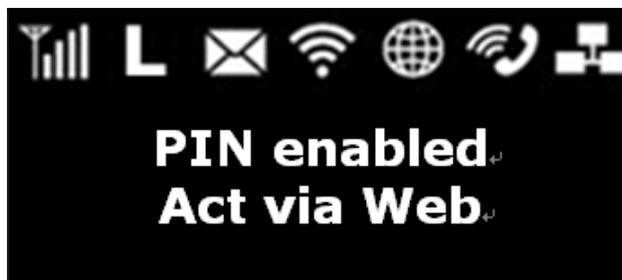
If the user has enabled the PIN security protection on the SIM card, the screen directs the user to access **4G LTE > PIN Verification** via the web interface before proceeding to use the Internet connectivity features of the device.
