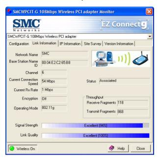
**Network Name** - This is the Service Set ID (SSID) for the wireless network to which you want to connect.
