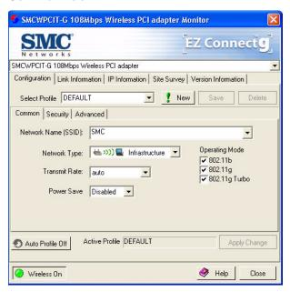
**Network Name (SSID)** — This is the Service Set ID (SSID) for the wireless network to which you want to connect.
