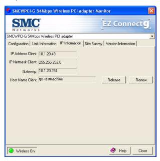
Now that you have configured your wireless adapter to connect to the wireless network, your adapter needs to obtain new network settings. By releasing old IP settings and renewing them with settings from the access point, you will also verify that the adapter is configured correctly.
