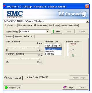
RTS Threshold - This sets the packet size threshold at which a Request to Send (RTS) signal must be sent to the receiving station prior to the sending station starting communications. Devices contending for the wireless medium may not be aware of each other. The RTS mechanism can solve this problem. The larger the threshold, the faster the speed.
