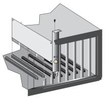
**Note:** Be careful that it does not touch any conducting parts on the computer motherboard.
