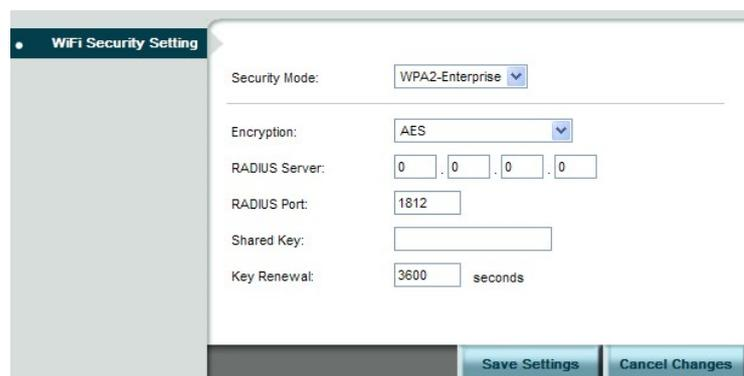
The screenshot shows the 'WiFi Security Setting' window. The 'Security Mode' is set to 'WPA2-Enterprise'. The 'Encryption' is set to 'AES'. The 'RADIUS Server' is set to '0.0.0.0'. The 'RADIUS Port' is set to '1812'. The 'Shared Key' is an empty text box. The 'Key Renewal' is set to '3600 seconds'. There are 'Save Settings' and 'Cancel Changes' buttons at the bottom right.
