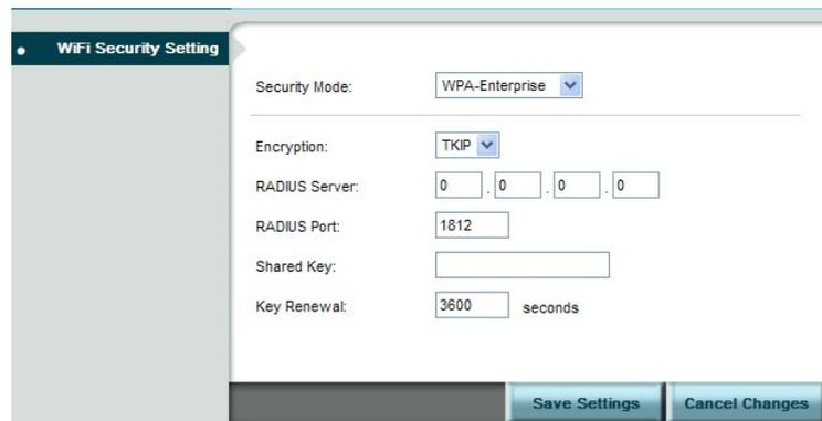
The screenshot shows the 'WiFi Security Setting' window. The 'Security Mode' is set to 'WPA-Enterprise'. The 'Encryption' is set to 'TKIP'. The 'RADIUS Server' is set to '0.0.0.0'. The 'RADIUS Port' is set to '1812'. The 'Shared Key' is an empty text box. The 'Key Renewal' is set to '3600 seconds'. There are 'Save Settings' and 'Cancel Changes' buttons at the bottom right.
