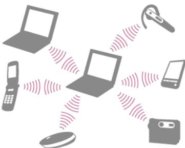
One BLUETOOTH device can connect with up to seven devices via wireless network to exchange data.
