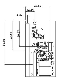
7.1.1 Top & Bottom View of CX Module with Bottom Shield
