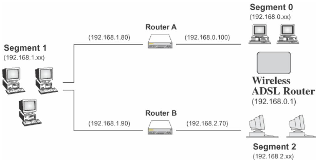
Figure 68: Routing Example
