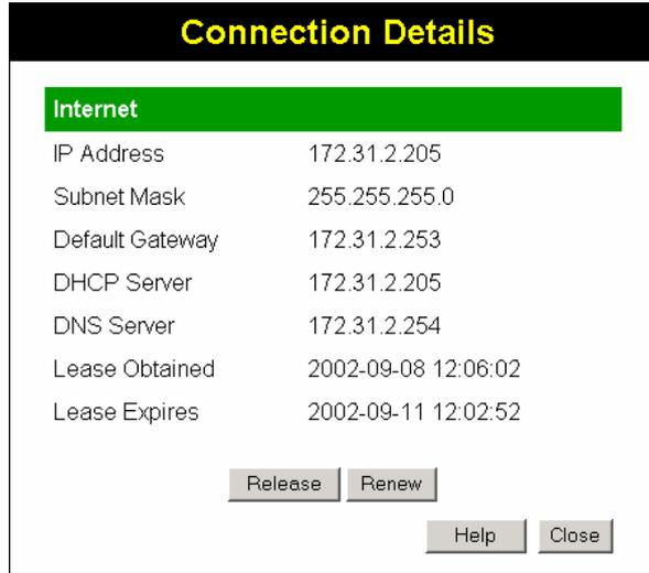
**Figure 50: Connection Details - Fixed/Dynamic IP Address**
