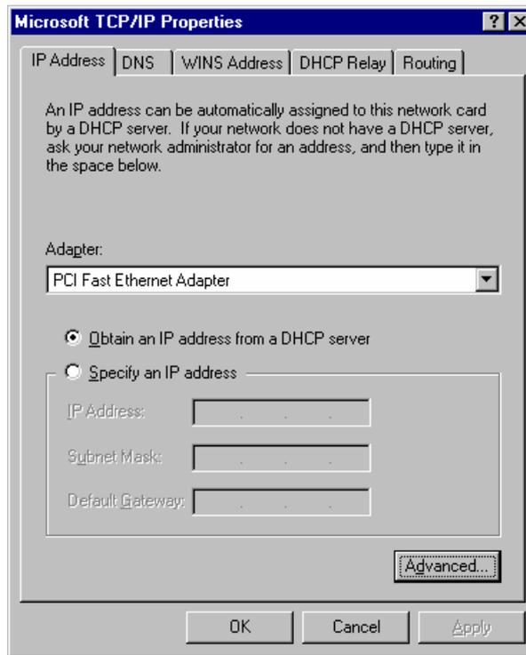
**Figure 26: Windows NT4.0 - IP Address**
