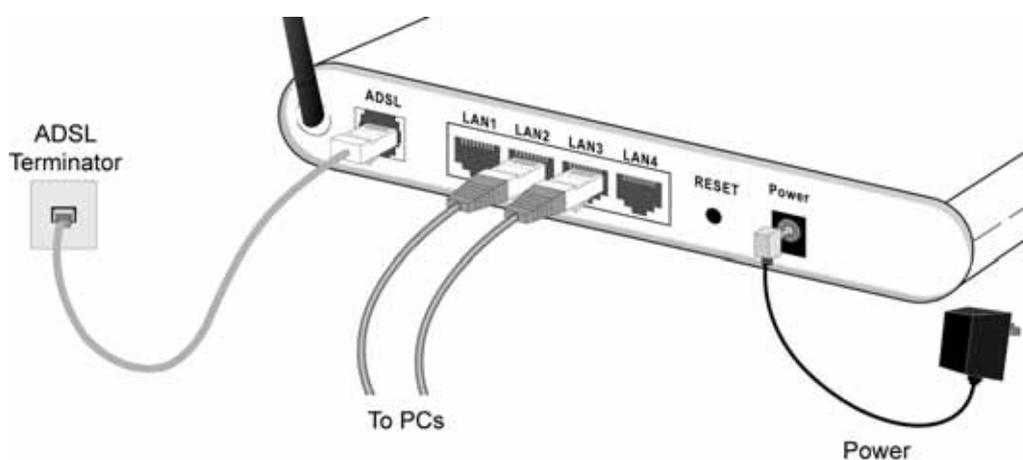
**Figure 4: Installation Diagram**
