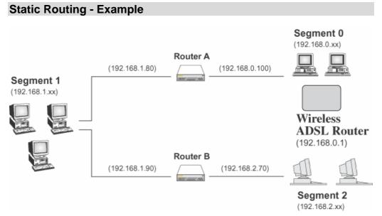
Figure 68: Routing Example
