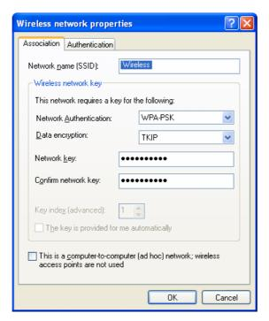
Figure 42: Wireless Network Properties- WPA-PSK
