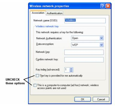
Figure 38: Wireless Network Properties - WEP
