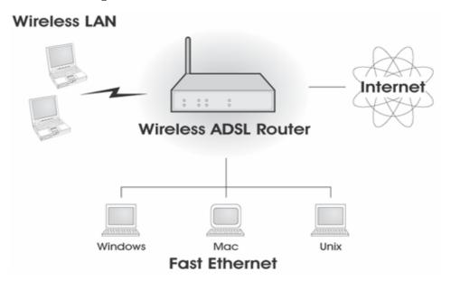
Figure 1: Wireless ADSL Router
