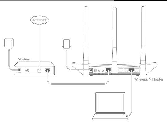
Figure 2-1 Hardware Installation
