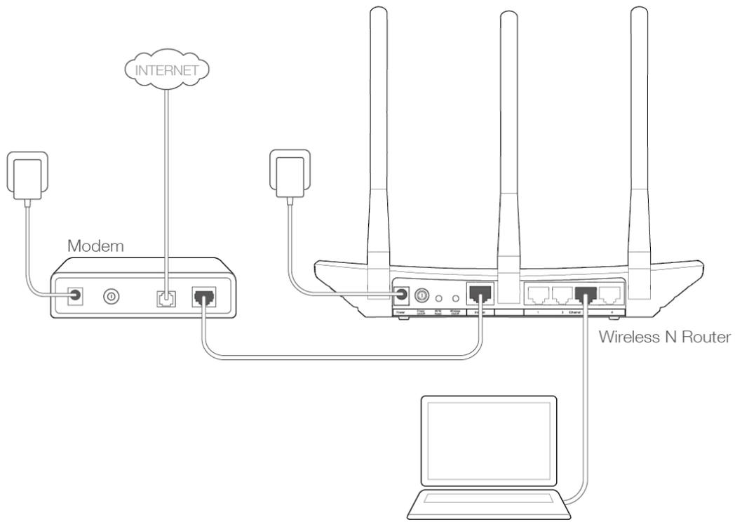
Figure 2-1 Hardware Installation
