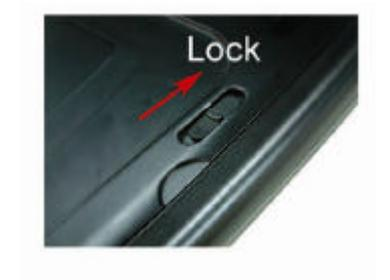
Release battery switch to lock it.
