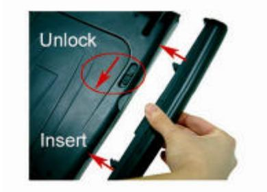
Unlock battery switch by pushing it downward.
