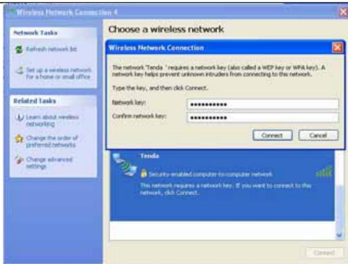
**Note:** If the wireless device to connect is not encrypted, the key dialogue box will not pop up.
