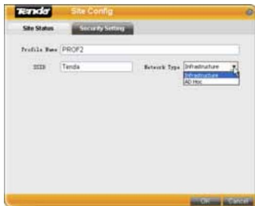
Infrastructure is a application mode which integrates the wired and wireless LAN architectures. What makes it different from Ad-Hoc is that the computer installed with the wireless network adapter has to fulfill wireless communication via AP or wireless router. It has "wireless AP + wireless network adapter" mode and "wireless router + wireless network adapter" mode.
