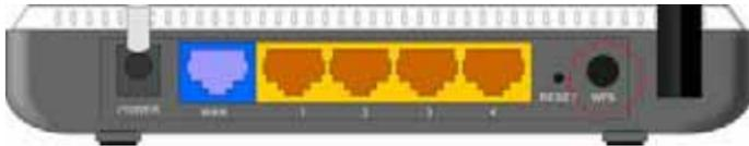
Keep pressing the WPS button on the Router's panel for one second if your wireless router supports WPS (such as Tenda W311R). The WPS indicator will keep flashing (for about 2 minutes). It indicates that the WPS function is enabled on the router. There are 2 ways to use wireless adapter for PBC connection:
