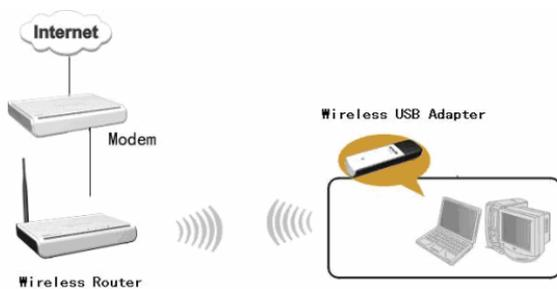
This wireless network adapter is a common solution for client signal reception.
