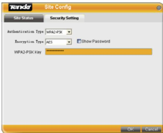
**Note:** If the wireless router or AP you want to connect closes SSID broadcast function, the wireless network adapter will not be able to scan this wireless network SSID. However, you can create the corresponding configuration file to connect.
