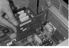
3. Fix the NIC with screws and cover the case.
