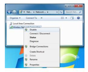
2. Attach the AP-3001g directly into a USB port on your PC. The AP3001g driver will auto run and install to your PC. A new wireless adapter "Wireless Network Connection" will show.
