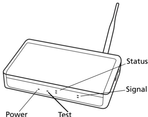
**POWER** – Indicates that the access point is receiving power from the power adapter.
