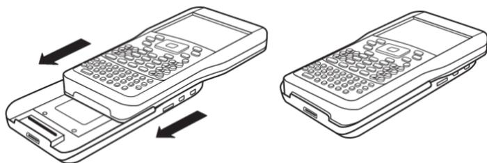
3. Press firmly to make a good connection. When properly connected, the TI-Nspire™ handheld appears to be sitting on top of the cradle.
