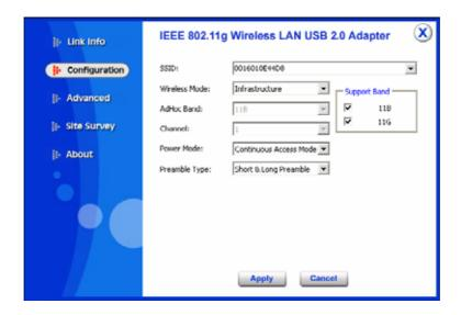
**SSID:** The SSID differentiates one Wireless LAN group name from another; so all access points and all devices attempting to connect to a specific Wireless LAN group name must use the same SSID. A device will not be permitted to join the BSS unless it can provide the unique SSID.
