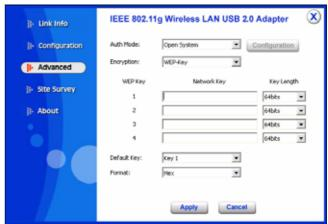
**Network Key:** Choose the encryption way, either in HEX or ASCII formats, and enter the password in the blank space.
