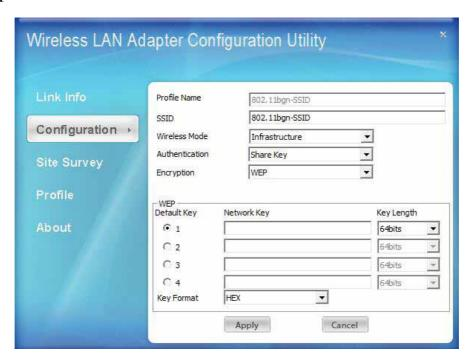
**Profile Name:** The default name is the same as the SSID of the platform which you connected and you can change the name you favor (the key length is limited  $1\sim32$  bits).
