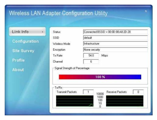
**Status:** Shows the associated BSSID, which can be used to identify the wireless access point.
