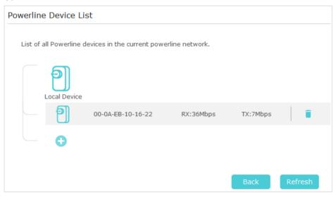
3. Click the add icon • and enter the Powerline Key of the device you want to add. The Powerline Key contains 16 capital letters, formed like XXXX-XXXX-XXXX. It is printed on the back of the powerline device.
