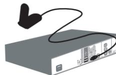
Plug the other end of the USB cable into one of the USB ports on the TiVo box. The power indicator (⏻) lights when the cable is connected.
