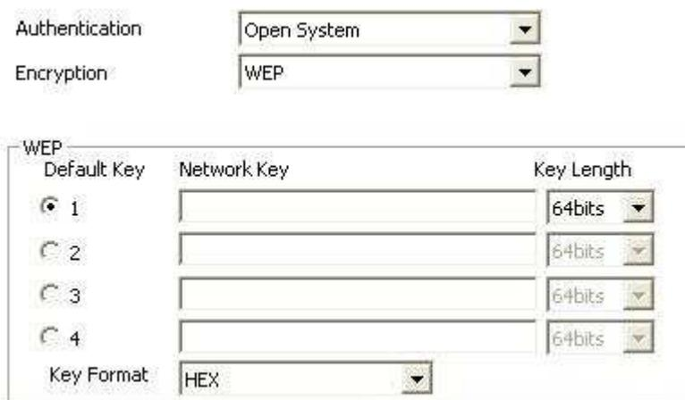
The screenshot shows a configuration interface for WEP. At the top, there are two dropdown menus: 'Authentication' set to 'Open System' and 'Encryption' set to 'WEP'. Below these is a section titled 'WEP' containing a table with four rows for 'Default Key' (radio buttons 1-4, with 1 selected), 'Network Key' (text input fields), and 'Key Length' (dropdown menus, all set to '64bits'). At the bottom of the WEP section is a 'Key Format' dropdown menu set to 'HEX'.
