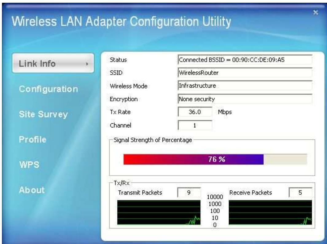
**Status:** Shows the associated BSSID, which can be used to identify the wireless access point.
