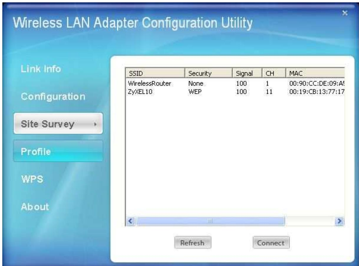
**Available Network** – displays the wireless networks (wireless clients and access points) that are within range.
