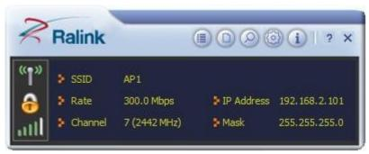
The Ralink wireless utility starts in compact mode as shown above, provides profile management, the available networks listing, a statistical counter display, Wi-Fi multimedia (WMM), protected Wi-Fi setup, Cisco compatible extensions (CCX), call admission control (CAC), radio controls, Ralink driver/utility information, and help
