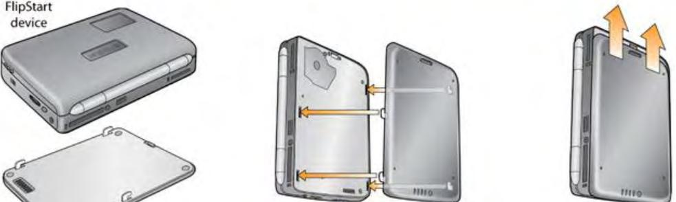
The diagram illustrates the process of attaching the battery in three stages. First, the FlipStart device and the battery are shown separately. Second, the battery tabs are inserted into the slots on the bottom of the device. Third, the battery is slid up into its locked position.
