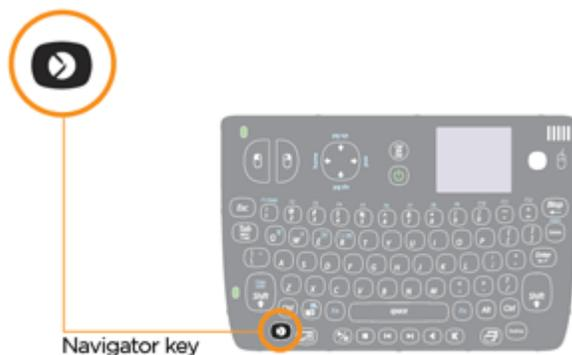
To show Navigator, press the Navigator key on the keyboard
