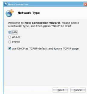
2. On the above menu, click the mouse to tick “LAN” and click the front panel of the item “use DHCP as TCP/IP default and ignore TCP/IP page” to cancel the tick, then click “Next” to enter the window of “TCP/IP Settings” as shown right:
