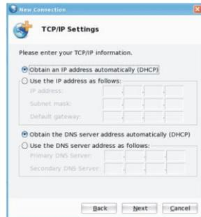
On the menu, you need to input the IP addresses, subnet masks, default gateway, DNS and etc, then click “Next” to enter the window of “Summary” to tick the item “connect after finish”, then the system will start connecting the network. After several seconds, click the icon
