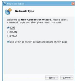
2. On the above menu, click the mouse to tick “LAN” and click the front panel of the item “use DHCP as TCP/IP default and ignore TCP/IP page” to cancel the tick, then click “Next” to enter the window of “TCP/IP Settings” as shown right:
