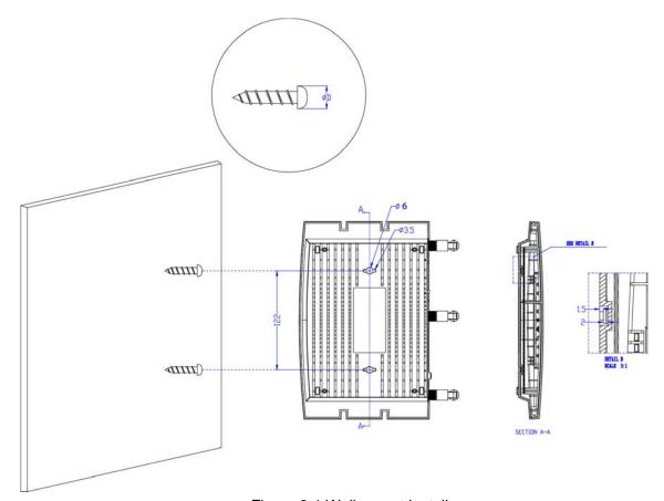
Figure 2-1 Wall-mount install
