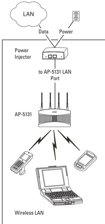
The Power Injector can be installed free standing, on an even horizontal surface or wall mounted using the power injector's wall mounting key holes. The following guidelines should be adhered to before cabling the Power Injector to an Ethernet source and an AP-5131:
