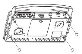
3. Attach the Radio 1 and/or Radio 2 antennas to their correct connectors. For information on the antennas available to the AP-5131, see "AP-5131 Antenna Options" on page 6.
