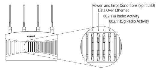
The five LEDs on the top housing of the AP-5131 are clearly visible in table-top, wall and below ceiling installations. The five AP-5131 top housing LEDs have the following display and functionality:
