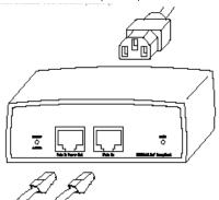
The Power Injector has no On/Off power switch. The Power Injector receives power and is ready for AP-5131 device connection and operation as soon as AC power is applied.
