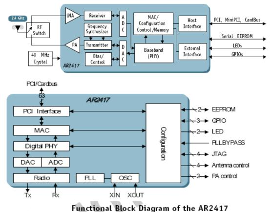
Processor : Atheros AR2417 single chip integrated with the MAC/baseband/radio Memory : Serial EEPROM:16K Antenna Interface :1x2.4G Dipole Antenna. I/O Interface : minpci
