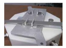
Hand tighten the Band-It strap through the pole mounting bracket, thread it through the strap buckle and then bend the strap back.
