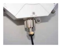
The following illustration shows a typical pole mounted XR-1000H installation after the antenna is installed and cable attachments have been completed.
