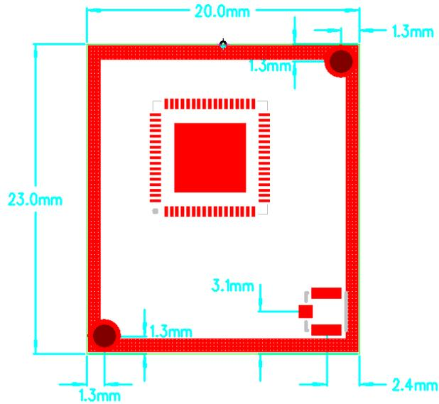
Fig 5.3.3 XG-182M Bottom View Drawing
