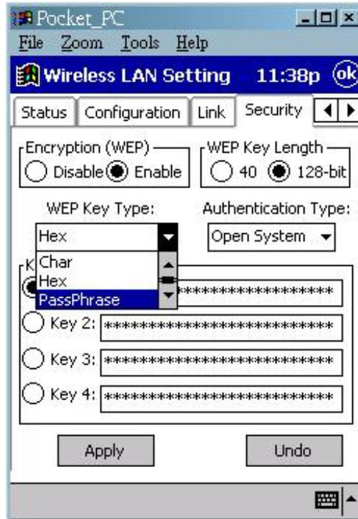
**Step 2.** Type a character string in the **Key in the phrase to generate keys** field, then click **OK**. As you type, the utility uses an algorithm to generate 4 keys automatically.
