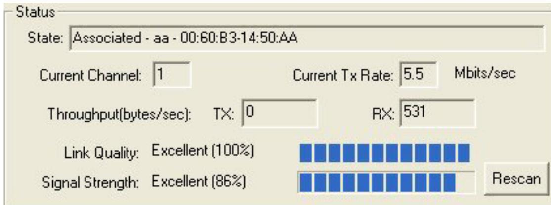
*State:* When operating in Infrastructure mode, this field shows the MAC address of the Access Point with which the Wireless LAN CF Card is communicating. When operating in Ad-Hoc mode, it shows the virtual MAC address used by computers participating in the Ad-Hoc network.
