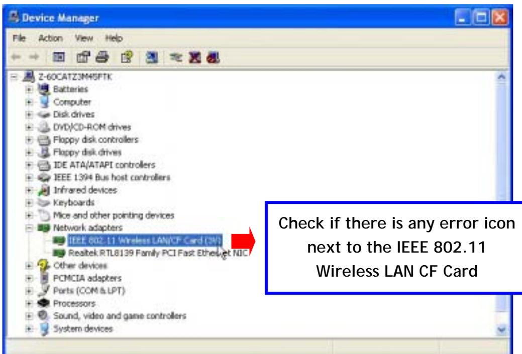
After installing the 11Mbps Wireless LAN CF Card, the Windows XP will display a “Wireless Network Connection #” message.
