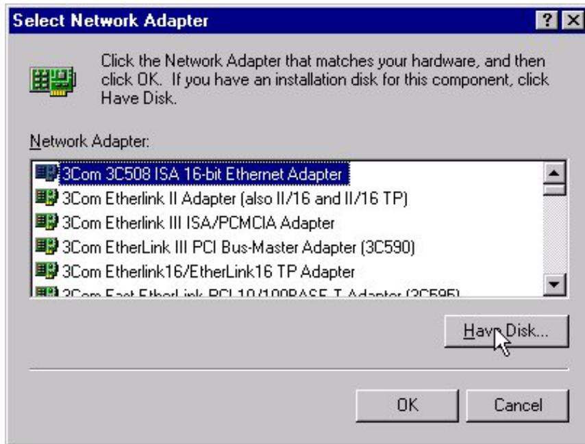
**Step 3:** Windows NT will ask for the path containing the 11Mbps Wireless LAN PC Card driver for Windows NT. Insert the Product CD-ROM into the CD-ROM drive, and then click **OK** to continue.
