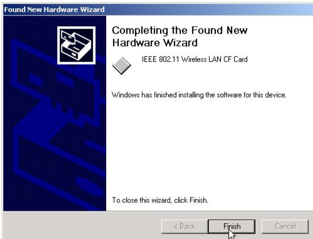
**Step 7:** Open **Control Panel/System/Device Manager**, and check **Network Adapters** to see if any error icon appears. If no, your 11Mbps Wireless LAN CF Card is working well.
