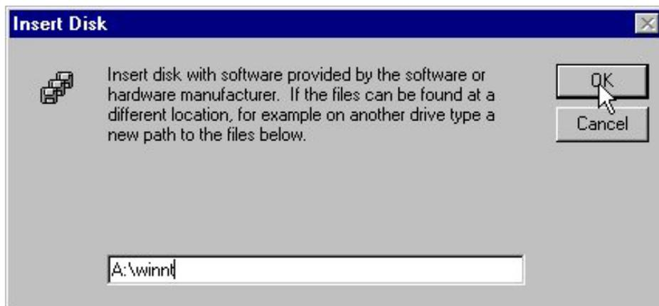
**Step 4:** The Windows will find “IEEE 802.11 Wireless LAN/CF Card”. Click **OK** and Windows will then copy the necessary files into the system.
