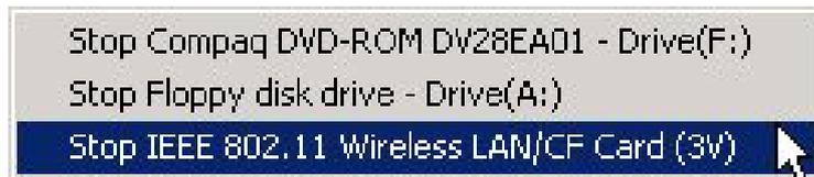
3. Wait a few seconds until the operating system displays a pop-up message to indicate you can safely remove the Wireless LAN CF Card. Click **OK** and you may then take out the 11Mbps Wireless LAN CF Card.
