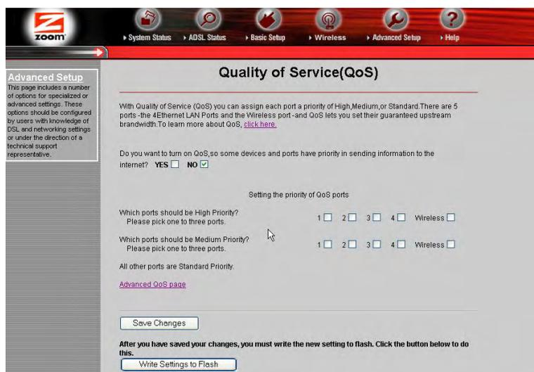
Note that on the QoS screen, Port 1 is the Ethernet port labeled LAN 1 on the X6 back panel. Port 2 is LAN 2, and so forth.
