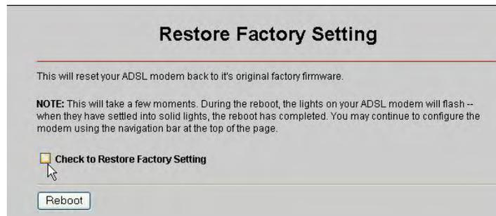
Follow the instructions on the page to reset your ADSL modem to its original firmware. Please see **Backing Up and Restoring Your Configurations** on page 91 for information about restoring a stored X6 configuration.
