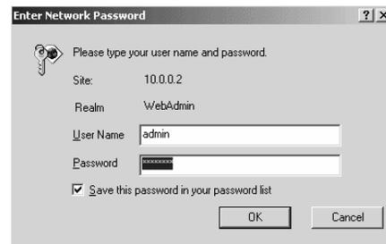
If you are not prompted for a **User Name** and **Password**, do the following in this order: Recheck all connections; restart the modem and computer; and reset the modem by inserting a paper clip into the **Reset** pinhole in the modem's back panel and press it three times.
