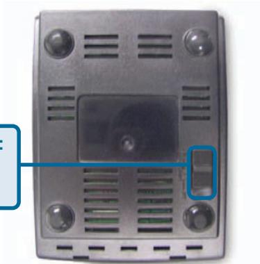
**Mode Selection Switch:** Used to select AP, client, or router mode.
