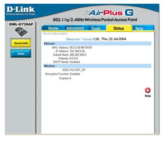
This screen displays the current firmware version, and the current wireless and Ethernet settings of the DWL-G730AP.
