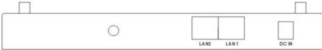
Figure 2-3 Side Panel of Bridge
