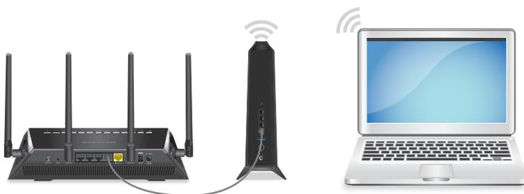
Figure 4. Extender in access point mode
