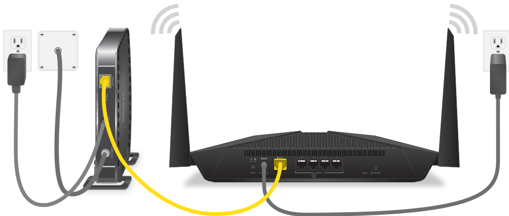
Figure 6. Cable your router
