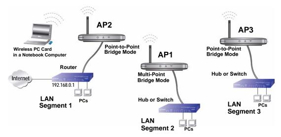
The following figure illustrates a multi-point bridge setup over three LAN segments.
