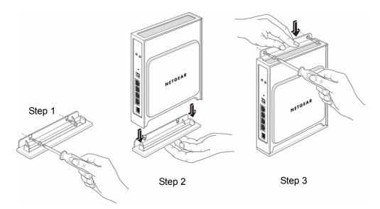
Figure 2-7 Installing the wall mount kit
