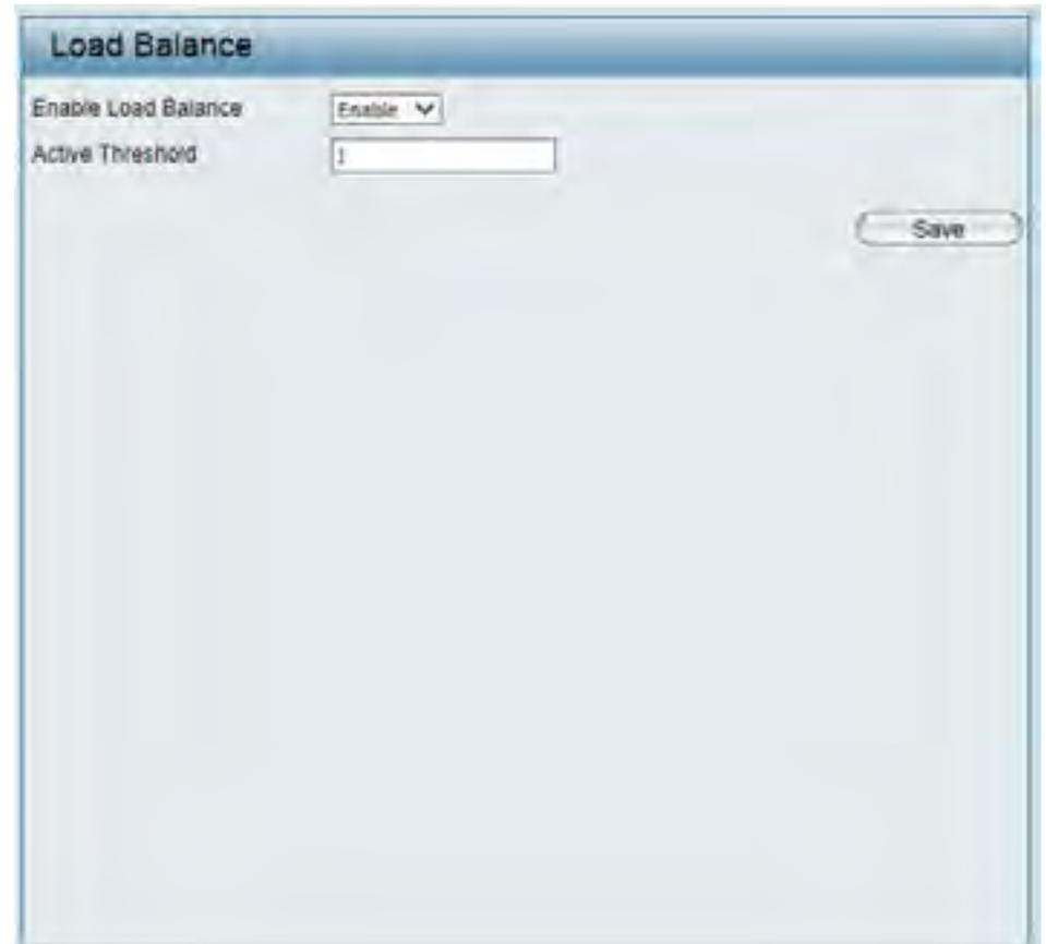
The screenshot shows a web-based configuration window titled "Load Balance". It contains two main settings: "Enable Load Balance" with a dropdown menu currently set to "Enable", and "Active Threshold" with a text input field containing the value "1". A "Save" button is located in the bottom right corner of the window.
