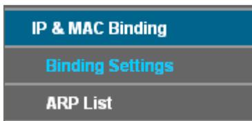
There are two submenus under the IP &MAC Binding menu: **Binding Settings** and **ARP List**. Click any of them, and you will be able to scan or configure the corresponding function. The detailed explanations for each submenu are provided below.
