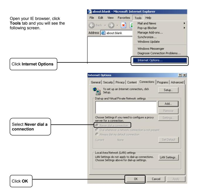
Now, try to log on to the Web-based configuration page again after the above settings have been configured. If you still cannot access the configuration page, please restore your modem router's factory default settings and reconfigure your modem router following the instructions in 3.2 Quick Installation Guide. Please contact our Technical Support if the problem still exists.
