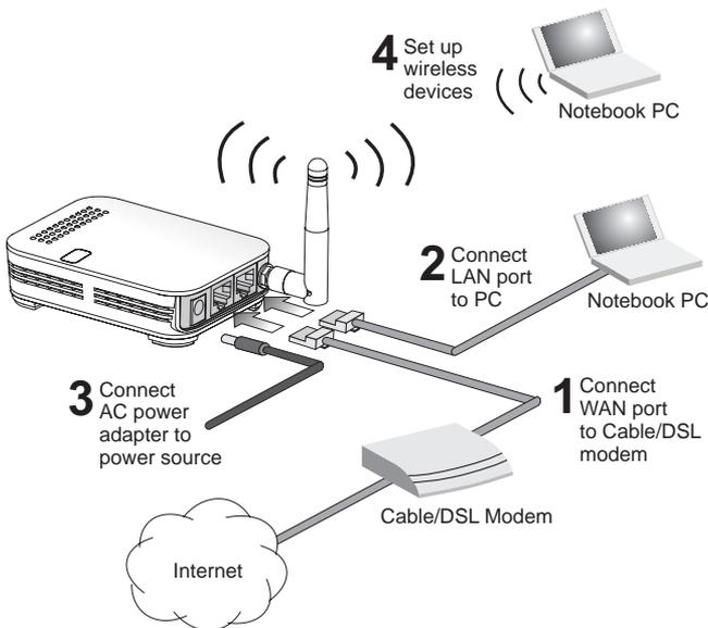
To connect the Mini AP Router in Router Mode for use as an Internet gateway, follow these steps:
