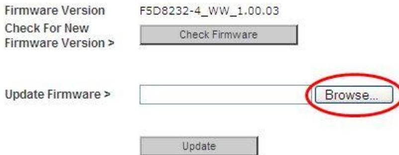
9. Select the firmware file by left-clicking on it and then click the “Open” button in the lower-right corner of the window. This will take you back into the Router's interface.
